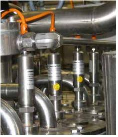
HYDROSTATIC LEVEL MEASUREMENT
