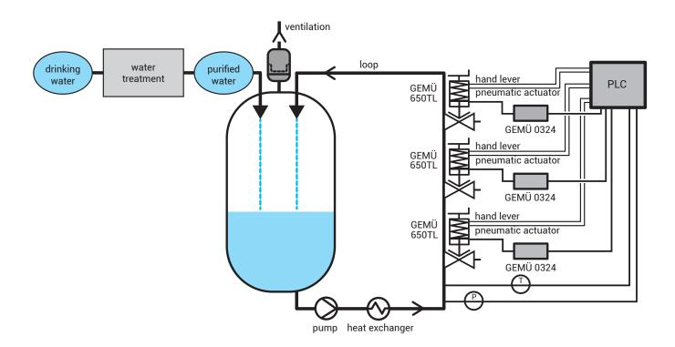
If the temperature is above the specified limit, the compressed air supply is interrupted for all valves which were previously opened manually and the valves move to in the closed position. However, the handwheel remains in the open position and must be turned clockwise manually to the closed position. This prevents the working medium from flowing out uncontrollably at the tapping points when the valve is pressurised again.
